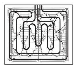
For grilling large quantities of thin cuts and for browning food in large dishes. The whole of the grill element is switched on. The inner part glows red. The outer part stays darker than the inner part but creates sufficient radiant heat for grilling.
